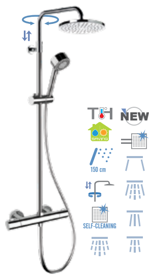
EQ 32 AMD20 CR € 552,60 Thermostatic shower mixer with upper 3/4" connection and lower connection 1/2" with integrated diverter, telescopic shower column, c.p. handshower 4 functions antilimestone, with 333 CNX 150 cm flexible hose and c.p. deluxe ABS shower head, rain jet, Ø 20 cm, with anti-limestone silicon jets.
