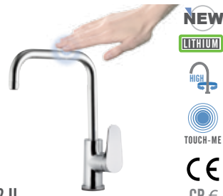
LT 72 U Single-lever sink mixer 90°, high squared "U" spout equipped with Touch-Me system with side lever and movable spout. Equipped with Ø35 cartridge.
