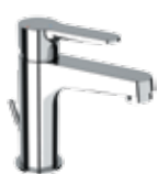
WE 10 LT8 CR € 78,70 Single-lever basin mixer with pop-up waste. Height 150 mm, interaxis 95 mm.
