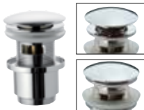
905 CC 2 € 29,90 Squared automatic pop-up waste 1"1/4 with click-clack system with overflow, model with shorter cup.
