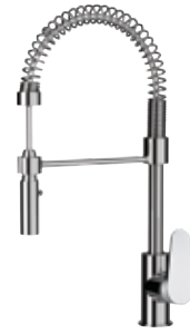
L 77 E Spring single-lever sink mixer with detachable and adjustable 2-functions hand shower and Ø 35 mm cartridge.
