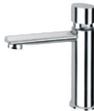
TE 22 Temporized tap 1/2", oval line all in Cp brass opening time 6-8 seconds.
