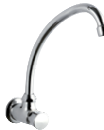
TE 42 Temporized (timer) upper mounted, with "J" spout, 1/2" tap, all in c.p. brass, opening time 6-8 seconds.
