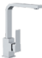
Q 10 G CR € 246,90 BO-NO € 395,10 Single-lever one-hole sink mixer, with short "U" spout, with squared click-clack waste with overflow. Height 280 mm, interaxis 180 mm.
