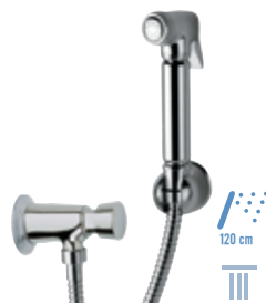
332 TEL CR € 74,50 Set composed of: shut-off hand shower, flexible cm 120, tempORIZED button flusher 1/2" all in C.P. brass, opening time 6-8 seconds.
