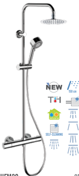
EQ32X UFM20 CR € 511,70 Thermostatic shower mixer with integrated diverter, upper 3/4" connection and lower 1/2" connection, minimal shower column, c.p. hand shower 4 functions anti-limestone, with 333 CNX 150 cm flexible hose and ultra slim stainless steel mirror polished shower head, Ø 20 cm, with anti-limestone silicon jets.
