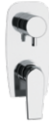
A 93 7 CR € 338,60 BO-NO € 541,80 Single lever built-in shower mixer with three ways diverter with seven positions (1 inlet and 3 outlets and seven positions to select single or mixed outlets) on single flange.
