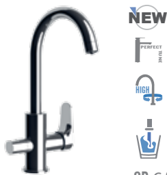
L 79 DW Three ways inlet single lever sink mixer, with movable spout and two fully independent outlets, with selection for drinking water directly from the lever.
