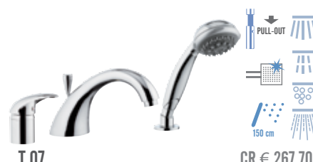
T 07 CR € 267,70 Single lever deck bath/shower mixer with integrated diverter on the spout, with heavy casted spout, anti-limestone pull-out hand shower 4 functions with hydro massage.
