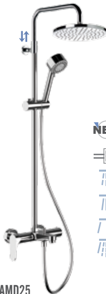
L34 AMD25 NEW CR € 477,50 Bath/shower mixer with upper 3/4" connection and lower 1/2" connection, with telescopic shower column, c.p. hand shower 4 functions antilimestone, with 333 CNX 150 cm flexible hose and minimal deluxe abs shower head Ø25 cm, with anti-limestone silicon jets.
