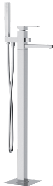
QD 08 CR € 1.219,30 Free standing bath mixer floor mounting with diverter and shower kit without waste. Height 900 mm, interaxis 223 mm.
