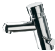
TE 19 M Temporized (timer) mixer with water mixing through headvalve, pillar tap with hot/cold water selection handle, serie minimal. 1/2", in c.p. brass, opening time 6-8 seconds.
