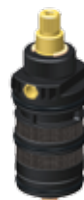
E 50 P Thermostatic cartridge with 330° angular handle rotation, 38° safety lock, working field from 5°C to 80°C, pressure field from 1 to 10 bar, stainless steel filter and safety system with the outlet lock in case there is one water lock, high performance thermoplastic materials.
