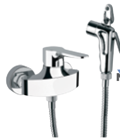
WC 31 DP Wall mounted single-lever shower mixer, interaxis 100 mm, with kit composed by shut-off hand shower in c.p. abs art. 332DPCR, conical flexible in c.p. brass cm 120 and c.p. hook art. 332GA.
