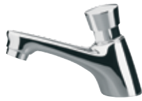
TE 15 Temporized (timer) pillar tap, 1/2", all in c.p. brass, opening time 6-8 seconds.
