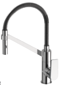
D 533 CR € 397,50 Single-lever mixer with black flexible hose coated with "fine design" spring, 360° movable, with detachable and adjustable 2-functions hand shower and Ø 35 mm cartridge.
